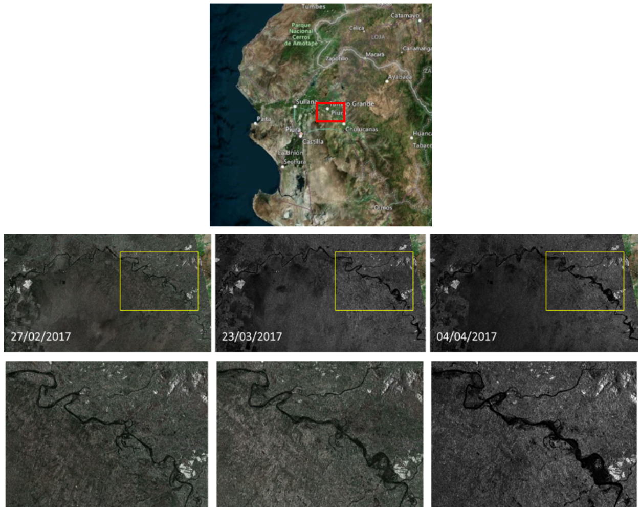
Figure 8 – Sentinel-1 (SAR) processed backscatter during the flood event 2017; generated by SatCen.
